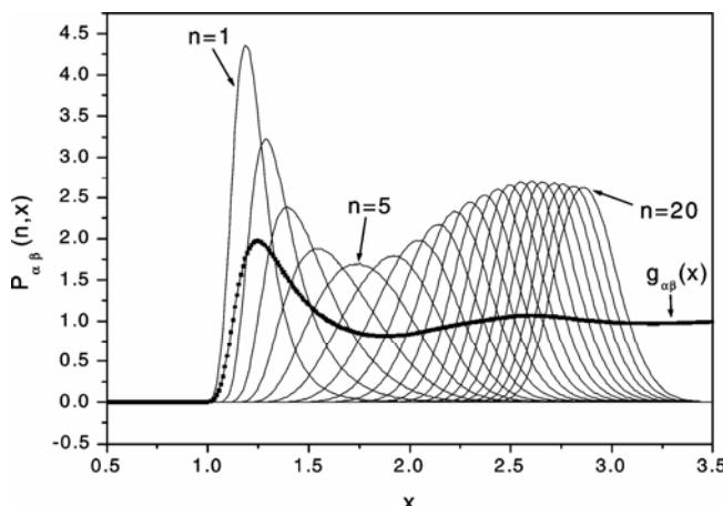
**Figure 5.**  $n$ th-NND functions for first 20  $\beta$ -type neighbours around a  $\alpha$ -type particle at the origin obtained from MD simulation for the binary mixture at  $\rho^* = 0.5$  at temperature mentioned in figure 1.
